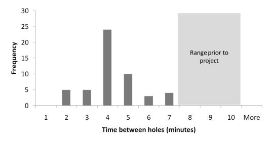
Figure 10. Improved charging cycle times due to automated blast loading (after Joseph, 2009)
