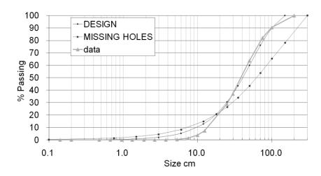
Figure 7. Effect of poor explosive distribution on fragmentation
