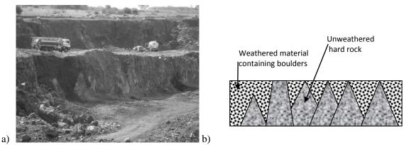
Figure 8. a) Photograph of top benches being charged and b) Schematic of rock cones interspersed with boulder material
