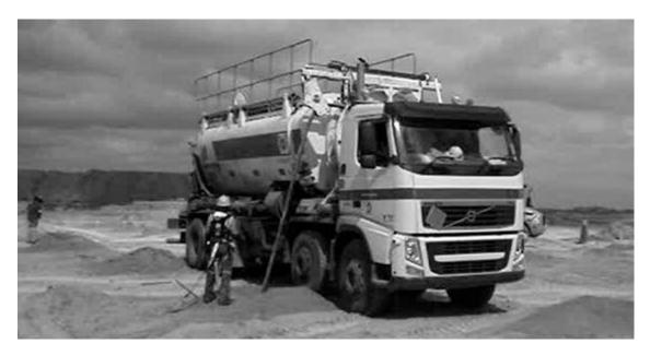
Figure 2. MMU and hose operator with GPS backpack
