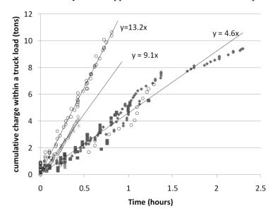
Figure 12. Plot of rate of explosive delivery for various benches logged
