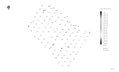
Figure 6. Explosive charge plan showing irregular pattern and missing holes
