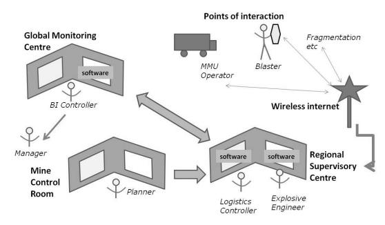
Figure 1. Schematic of Blast-i<sup>TM</sup> blasting intelligence system
