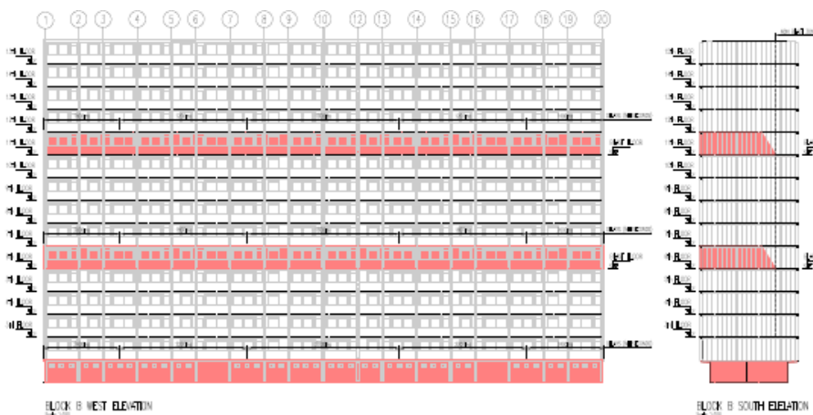
Principle of blast design showing the blast floors.
