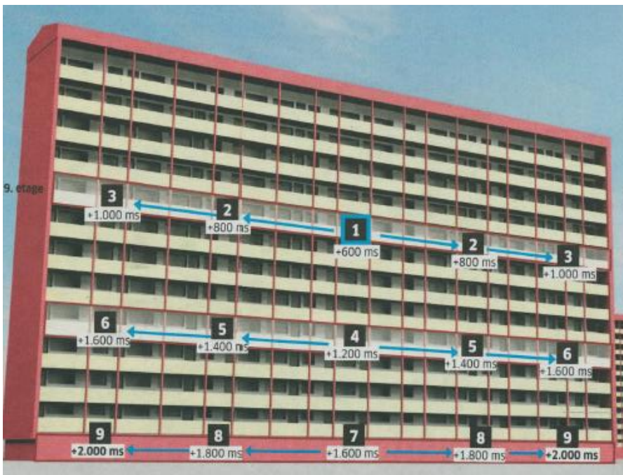
Principles of blast design showing the time delays of blast sequence, from step 1 (600 ms) to step 9 (2000 ms)
