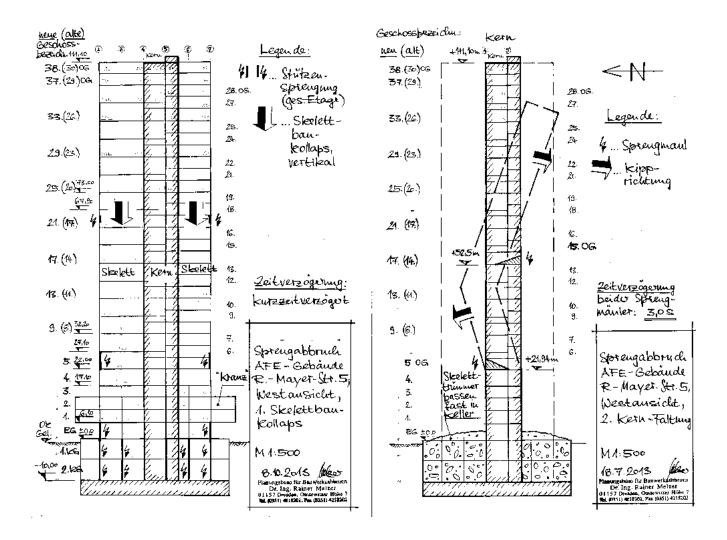
On the contrary in the blast mouth charges were placed about 400 electronic detonators. The three second time displacement was decided so that dropping slabs were sheltering the upper core blast mouth in its detonation yet. Water filled "big bags" on the roof should help to control the dust. To the blast a 250 m exclusion zone was established around the tower.
