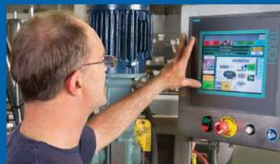
HMI touch screen control makes operation and performance analysis easy and intuitive.
