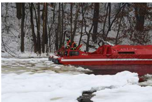
Breaking of ice barriers by a floating rescue tank or a mobile excavator
