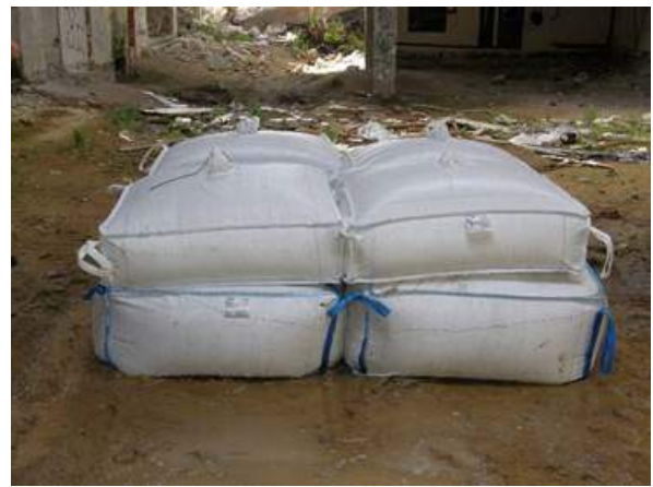
Two layers of 250 l bags (top) and 500 l bags (bottom) -The square base
