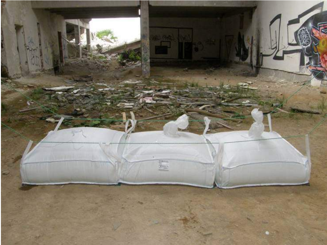
250 l bags hanging on pre-tensioned flexible ropes
