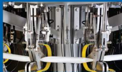
Reliable packaging of sealed and clipped chubs at production rates over 330 pieces per minute.
