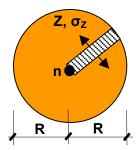
Figure 4, Cylindrical blasting model (length: 1 m)
