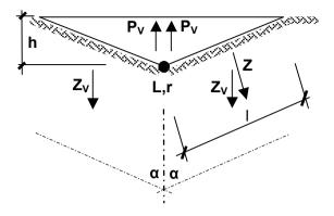
Figure 6, Wedge blasting model (1 m length)
