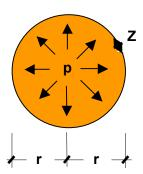
Figure 2, Explosive cylinder (length: 1 m) with tensile ring force **Z** [MN/m]
