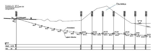
Sample of borehole alignment
