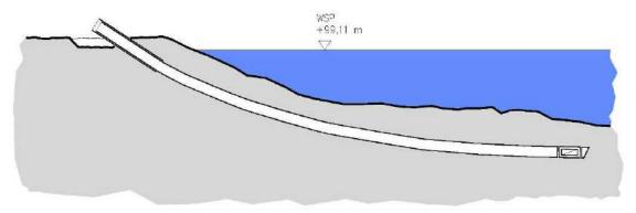
Drilling of the blast holes with HDD technique and surveying tool
