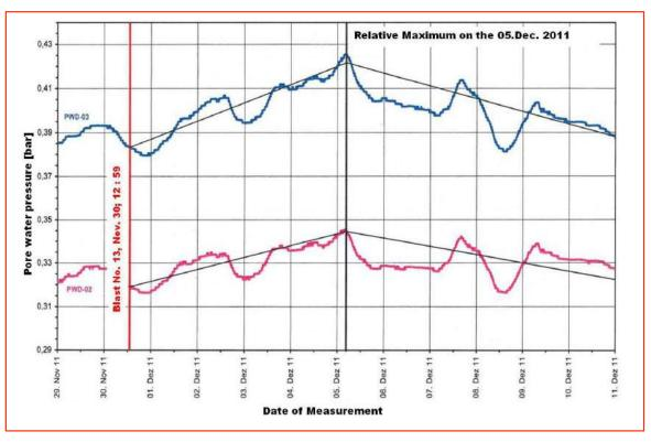
Pore water pressures after blast No. 13 (distance to blast: Transducer 2: 1450 m/4757 ft, Transducer 3: 1400 m/4593ft)
