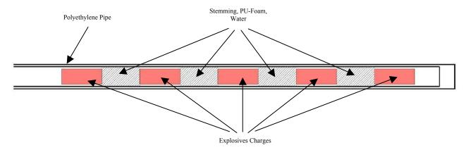
Blasting Pipe with up to 14 decks/charges (Austin Powder)
