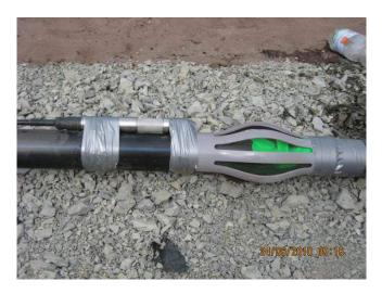
Pore water pressure transducer prepared to use in horizontal drill holes (Test 1 und 2)
