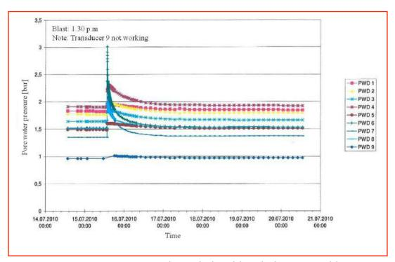
Pore water pressure measured 5 m below blast holes at test blast 2
