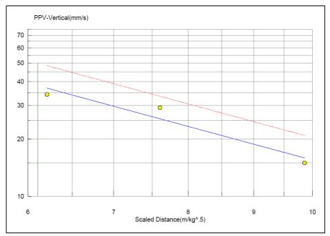
Figure 2. Regression Analysis of test blasts
