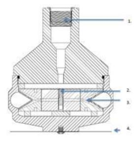
1. Threaded top connection (to cable head/ shock absorber). 2. Initiation Point. 3. Shaped Charge. 4. Centralizer.
