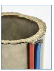
Tubular cutters for casing and control lines.
