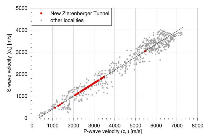
Fig. 5: Correlation between P- and S-wave velocities (red = clay siltstones from Zierenberg Tunnel)
