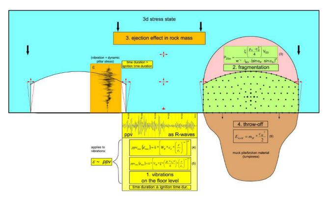
Fig. 12: Four-phase model of 3-D blasting underground
