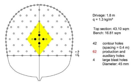
Fig. 15: Drill pattern for drill and blast with a blasting pull of 1.80m and q = 1.3 kg/m^3  $\,$
