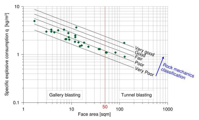
Fig. 13: Graph used to estimate the specific explosive consumption q (in kg/m<sup>3</sup>) depending on the face area and excavation strength [after 7]
