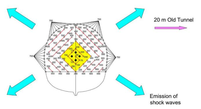
Fig. 18: Firing sequence in the roof section with spiral cut and simultaneous detonation in the auxiliary holes (figures indicate rounds of non-electric detonators at the bottom of boreholes)
