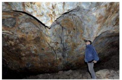
Fig. 5. Rabenstein Hodruša-Hámre – example of extraction by fire setting
