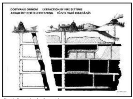
Fig. 4. Extraction by fire setting
