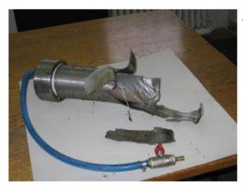
Fig. 6.1. State of cylinder no.1 after testing
