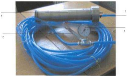
Fig. 5. Full system for testing of the resistance to hydrostatic to pressure of civil use explosives
