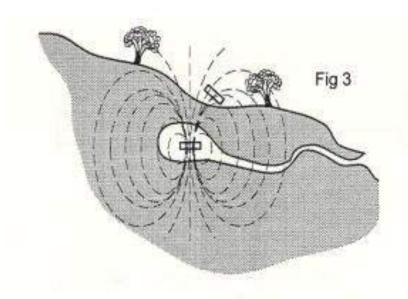
An assistant then walks away from the loop in a line that is in the plane of the vertical loop. At a reasonable distance, say 15 metres, a second marker pole is placed in the ground. This line between the two poles is the first of
