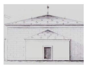
Fig. 12. Powder storage with lightning conductor
