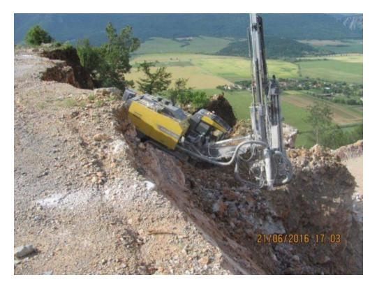
The drilling machine was approximately 5 meters below the level of the bench IV, on an inclined position, it leans on a rock and seems to be on a stabilized position.
