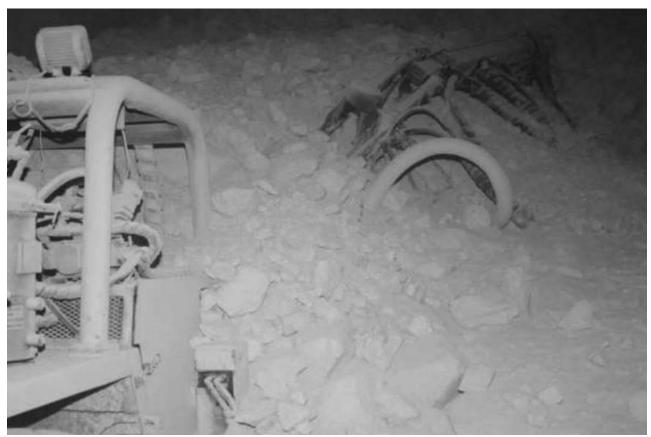
Figure 5. Underground vehicle at SLC mine after an inflow
