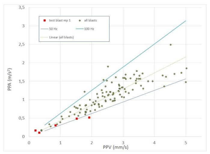
Figure 7.3 The relation between PPV and PPA. The lowest line shows the predicted line (50 Hz) corresponding to the test blast (red squares), while it can be seen that the actual relation between PPV and PPA varies between 50 and 100 HZ averaging at 67 Hz (the dotted line)
