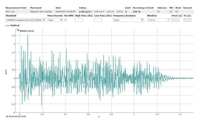
Figure 6.3. Waveform of the acceleration from blast 92
