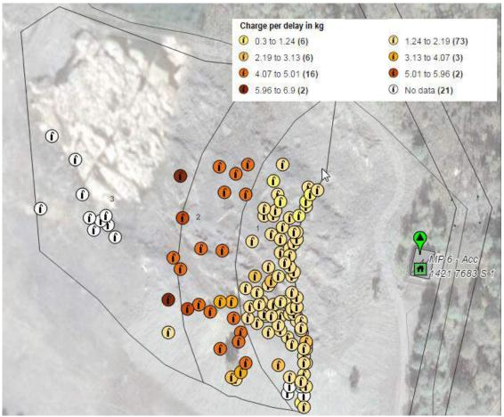
Figure 6.2 Location of the 120 production blasts. Charge per delay is shown with different colours accordingly to the legend in the figure
