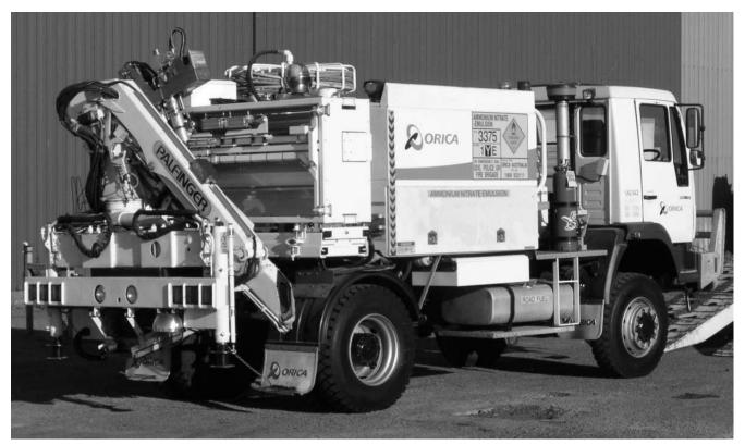
Figure 9. Early remote-control charging equipment with smart vision systems to identify blastholes
