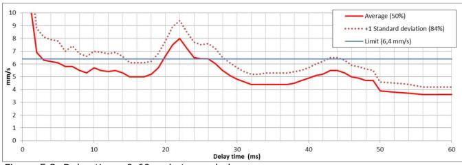
Figure 5.3. Delay times 0-60ms between holes
