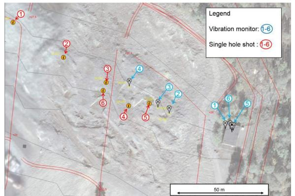
Figure 3.1. Map presenting 6 single shots in red and 6 vibration monitors in blue. The substation is the grey building on the right side of the map
