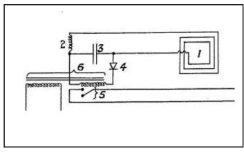
Figure 1. An image illustrating the wireless receiver from an early patent for a directly initiated detonator
