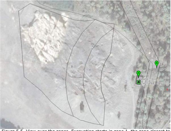
Figure 5.5. View over the zones. Excavation starts in zone 1, the zone closest to the substation (MP 6)
