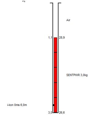
Figure 5.2. Charged bore hole, 3 kg charge, 3.5 m depth
