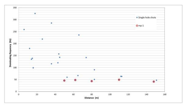
Figure 4.3. Dominating frequency verses distance, the red circles comes from MP1 at the substation
