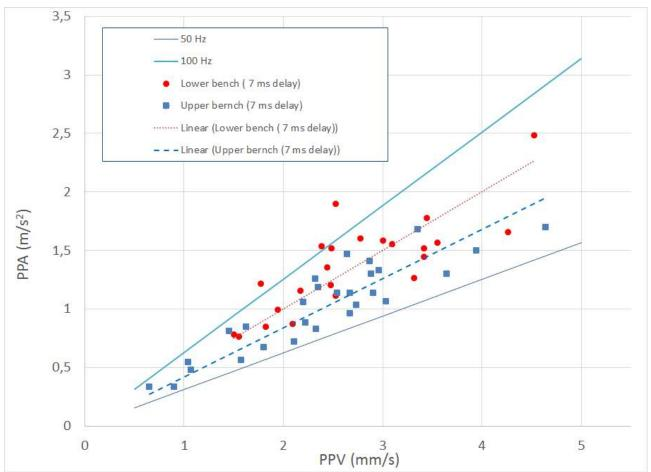
Figure 7.4 The relation between PPV and PPA. For just the 7ms delay shot. The upper bench (blue squares) gives an average frequency of 67 Hz while the lower bench (red circles) gives 80 Hz
