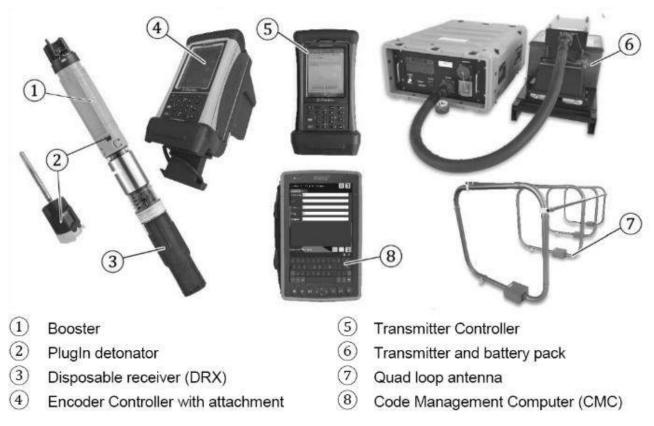
Figure 3. WebGen<sup>™</sup> 100 blasting system
