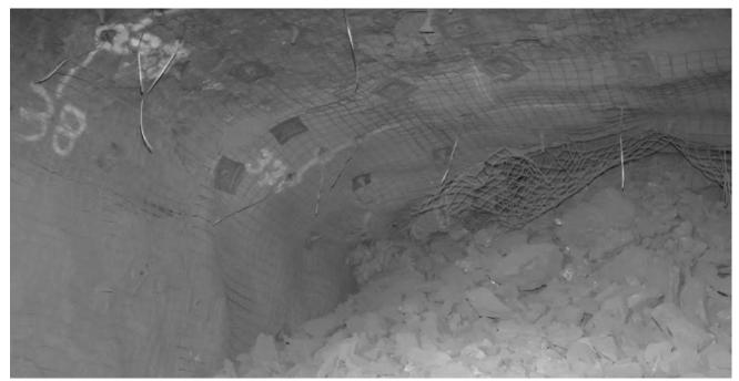
Figure 7. Multiple wireless charged rings are ready to fire as soon as needed, note strapping indicators
