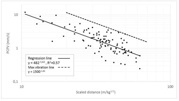
Figure 6. Principal component particle velocity (PCPV) versus scaled distance. The data points are randomly generated and not measured.
