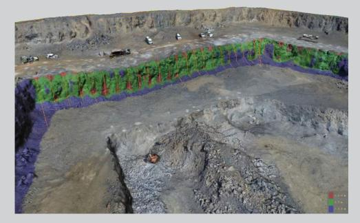
3D images from drones are a perfect survey of large blast sites. Poor blasting results are often caused by inaccuracy of the front row hole placement and suboptimal blast pattern geometry.
