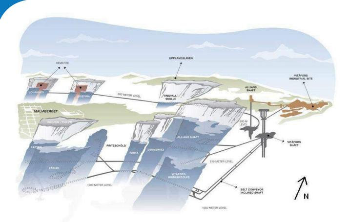
Figure 1. Schematic view of the orebodies at Malmberget Mine.
