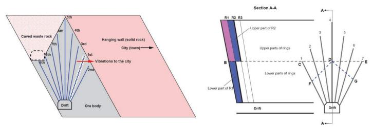
Figure 4. Changed initiation sequence (left) and divided ring blasting (right), from Zhang (2012).
