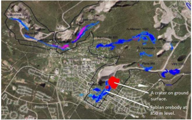
Figure 2. Aerial view of the Malmberget Mine site. Colored objects are horizontal projections of the orebodies at a specific level shown above.
