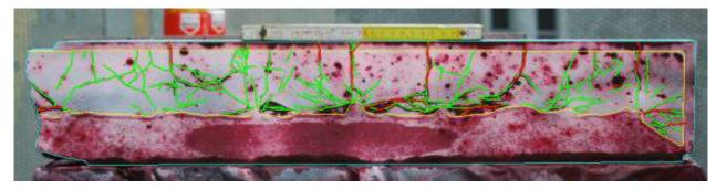
FIG 5 -Surface crack detection in cut slices
