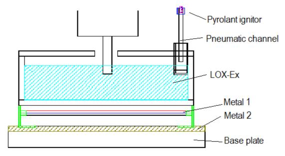
Pic. 12: Example of a filled explosion arrangement
