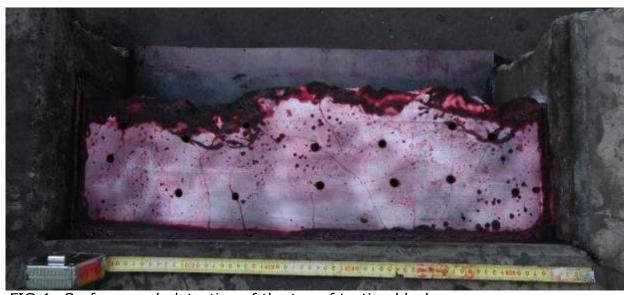
FIG 4 -Surface crack detection of the top of testing blocks
