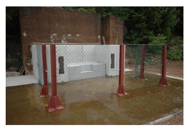
Figure 1 –Yokes at the Erzberg blasting site. They allow waves to escape from a test specimen. The inner yoke has room for the block.
