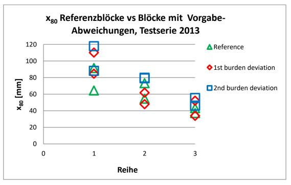
FIG 9 –Percentile size x<sub>80</sub> values, plotted row wise for blocks shot in 2013
