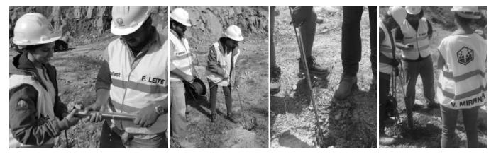
Figure 7. Field Procedure from left to right: probe assembling; probe deployment; offset measurement; measurement time record
