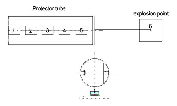
Pic. 11: Scheme of an automated explosion production facility with LOX-Ex
