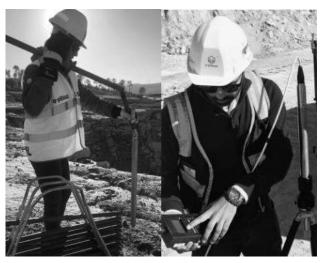
Figure 2. Rodded Boretrak (left) and Cable Boretrak (right)
