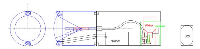
Pic. 9: Modules of the LOX-Ex method integrated in tunnel boring machine
