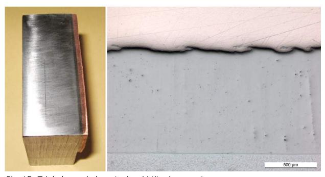
Pic. 15: Triple layer; below steel; mid titanium; on top copper
