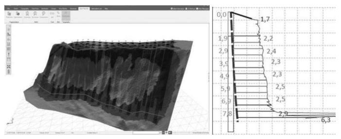
Figure 4. Critical Burden Detection (O-Pitblast)
