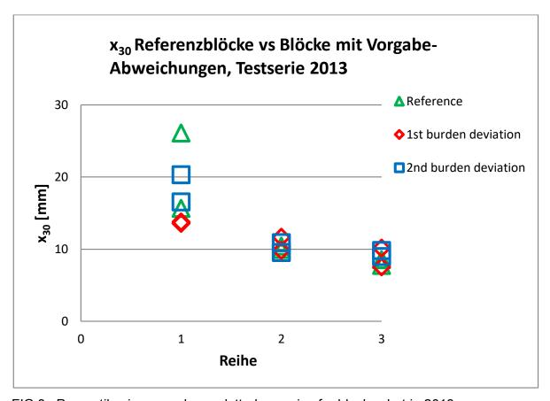
FIG 8 –Percentile size x<sub>30</sub> values, plotted row wise for blocks shot in 2013
