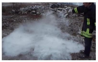
Pic. 5: Disposal of PMMA-LOX-Ex; here approx. 300 g
