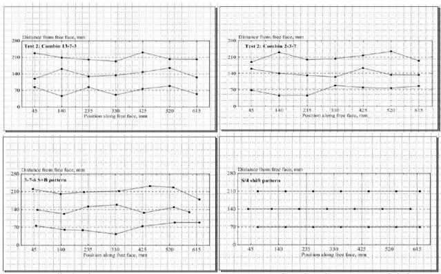
FIG 3 –Drilhole deviation patterns: Top 2013: 13-7-3 (1st burden variation) left and 2-3-7 (2nd burden variation) right; Bottom 2014: 3-7-6 (S+B deviations) left and S/4 shift right
