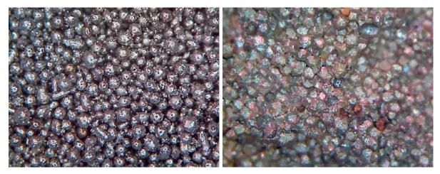
Pic. 16: Stellite granules on steel; left before, right after explosion
