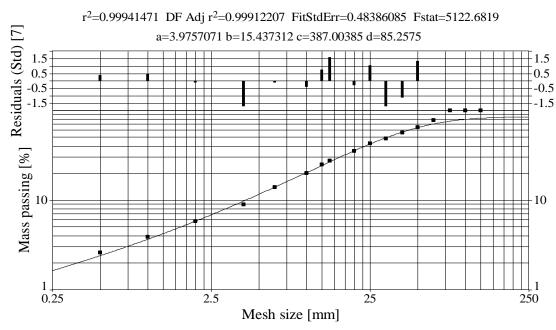
FIG 7 -Sieving curve block CH01B04 (1st burden deviation)
