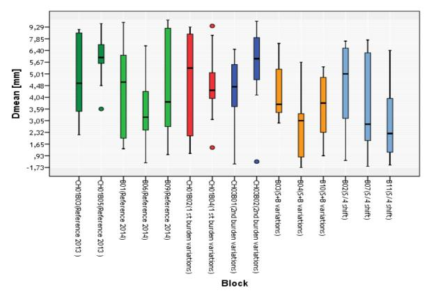
FIG 15 -Box- Whisker plot over the surface roughness Dmean for different drill patterns
