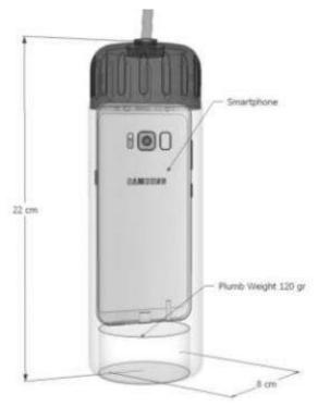
Figure 3. Smartphone used to measure holes
