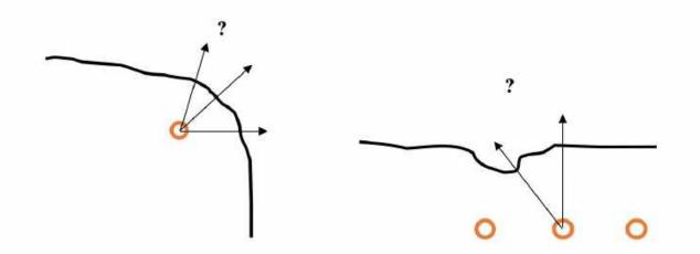
Figure 3. In which direction shall the profile measure in case of a corner hole (left) or a face irregularity (right)?
