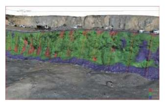
Figure 6: Minimum burden chart with indicated location of boreholes; green colour shows design burden, red: light burden, and blue: heavy burden
