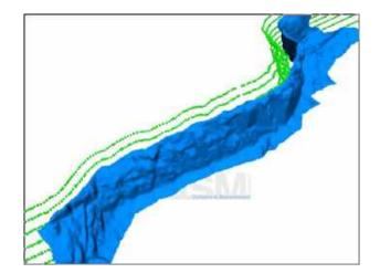
Figure 7. The computation of the minimum burden surface starts with the determination of according sample points (green)
