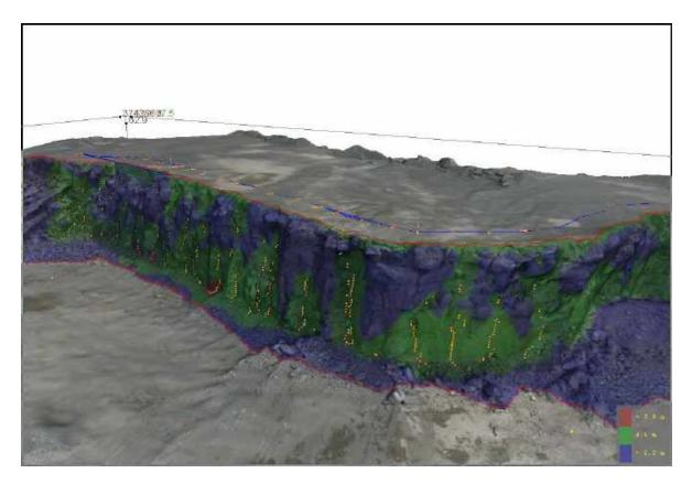
Figure 9. Minimum burden chart for automatically placed boreholes on a curved corner blast; bright dots indicate locations of minimal burden.
