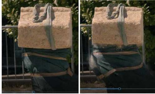
Figure 16. Protection against debris and fly rocks (record of high speed camera)
