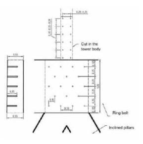
Fig. 7. Blasting holes position on ring belt and cuts.
