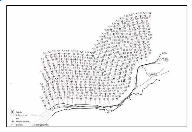
Figure 10. Automatically placed boreholes with loose constraints in azimuth and inclination
