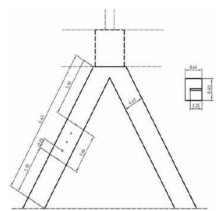
Fig. 6. Blasting holes position on inclined pillars.
