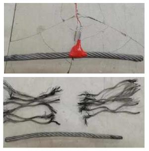
Figure 12. Wire rope explosive cutting test
