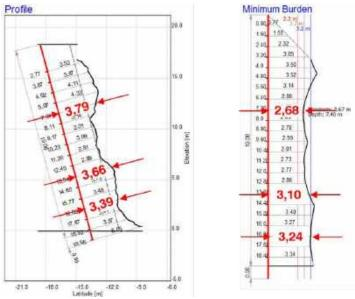
Figure 5. Profile and minimum burden diagram for the same borehole; note the significant differences at the indicated hole depths
