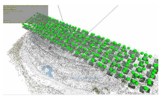
Figure 2. Analysis of deviations between camera locations from GPS recording (spheres) and photogrammetry-determined (pyramids).
