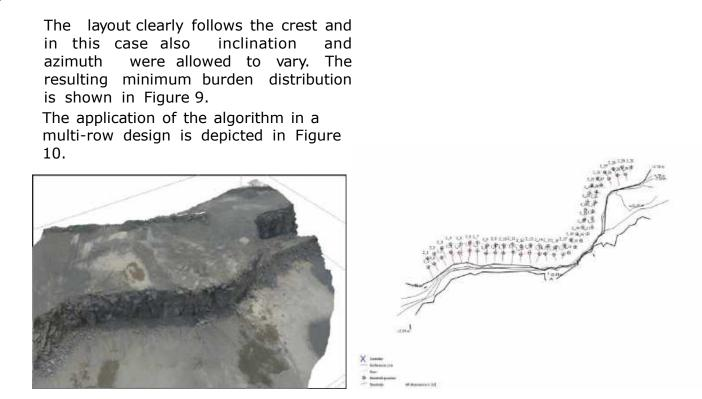
Figure 8. Left: 3D image of a curved blast site; right: plan view of automatically placed boreholes using minimum burden surfaces; the boreholes follow the crest
