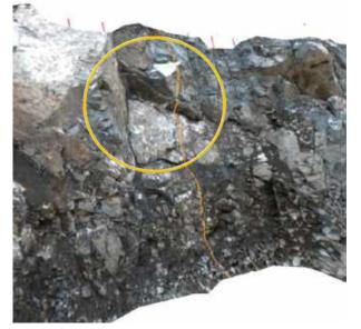
Figure 4. 3D model with a single profile; circle marks an irregularity (remainder of a detached block)
