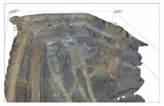
Figure 1. Comprehensive 3D model of a blast site and adjacent area
