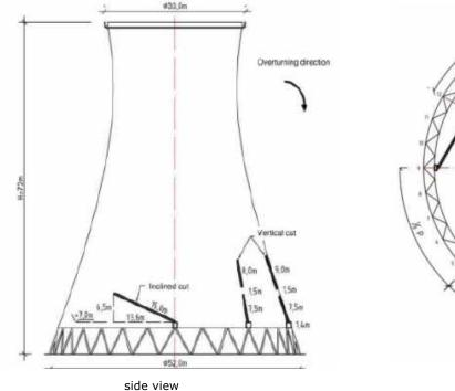
Fig. 5. Location of the cuts on tower body.
