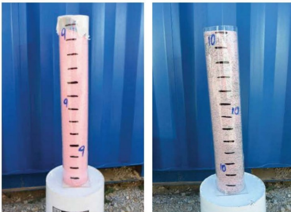
Figure 1. ANFO charge with 9% of water and ANFO with 4% of Al
