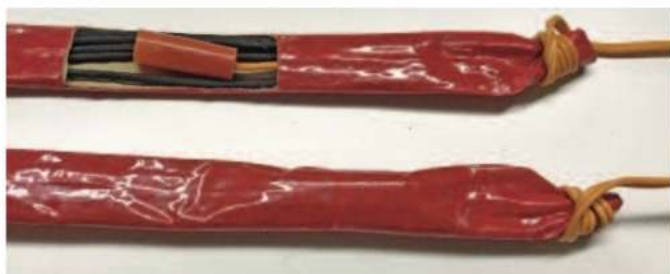
Figure 9. Electric Igniter sitting inside the fuse with the shroud in place.
