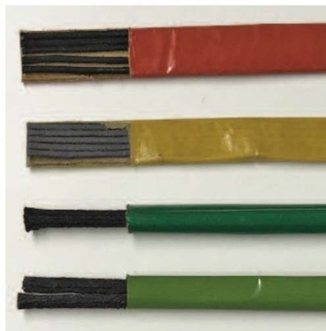
Figure 2. four varieties of quickmatch. from the top; 5 strand black powder, 5 strand perchlorate, single strand black powder and double strand black powder.
