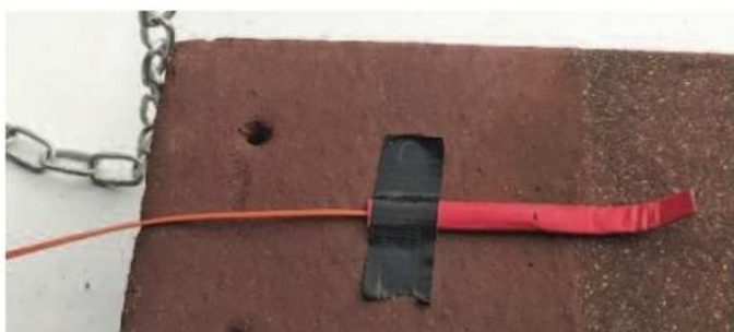
Figure 14. 100mm strip of fuse with electric igniter inserted ready for testing.
