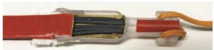
Figure 8. cut through showing position of Electric igniter in relation to fuse composition.
