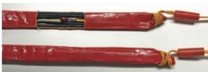
Figure 10. Electric igniter sitting inside the fuse with the shroud removed.
