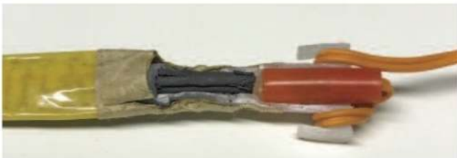
Figure 6. cut through showing position of Electric igniter in relation to fuse composition.
