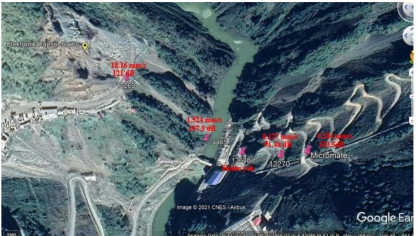
Figure 8. Display of vibration and air shock values measured from seismographs on Google Earth
