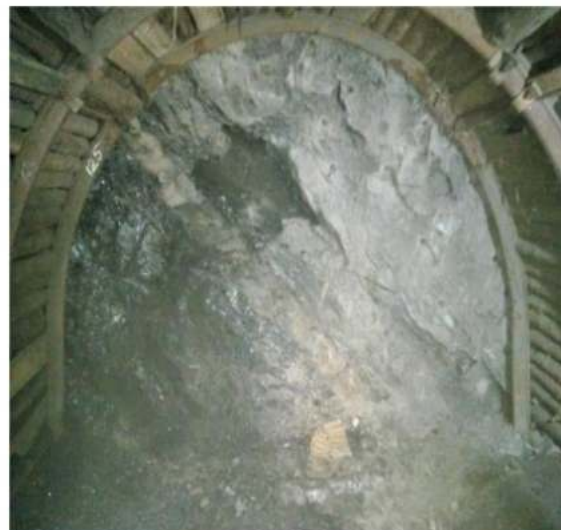
Fig. 6 Directional gallery in mixed coal & rock face, before and after blasting
